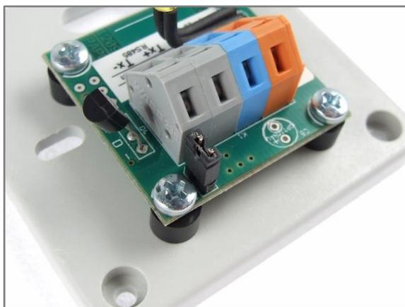
*fig. 3 - if the setup jumper is shorted, TQS3 communicates via ModBus RTU*
