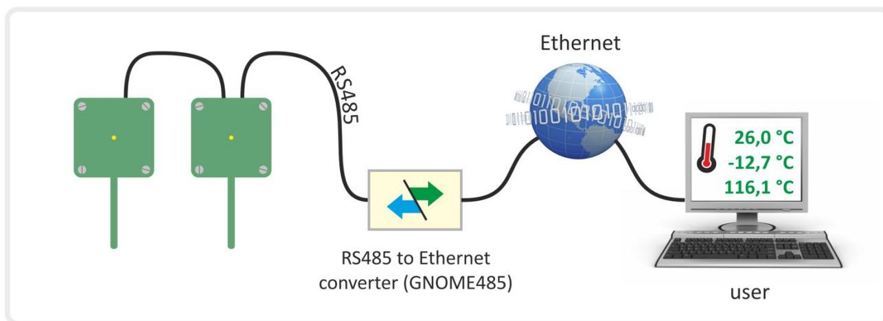
The module measures temperature using an integrated unit with the accuracy of  $\pm 0,5^{\circ}\text{C}$ . The TQS3 module contains an indicator which blinks to signalize the ongoing temperature measurement.
